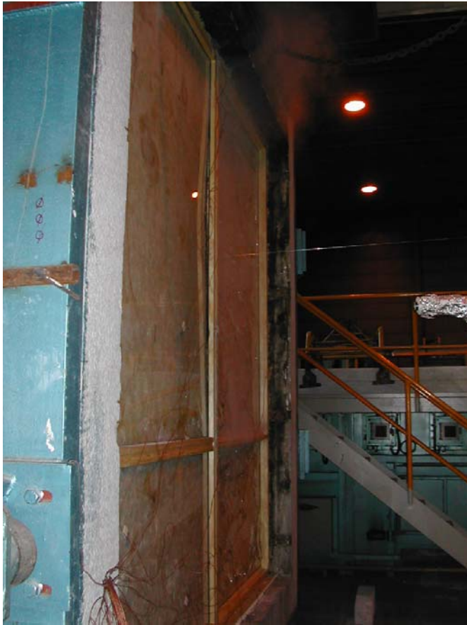
Photo 9: Unexposed side of the test specimen. The glass bends into furnace and have a displacement from flange.
