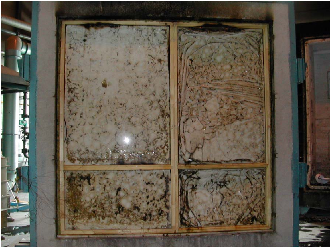
Photo 7: Unexposed side of the test specimen after test.
