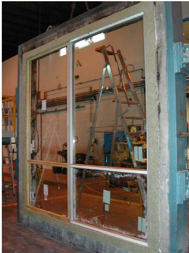
Photo 1: Exposed side of the test specimen before the fire test.
