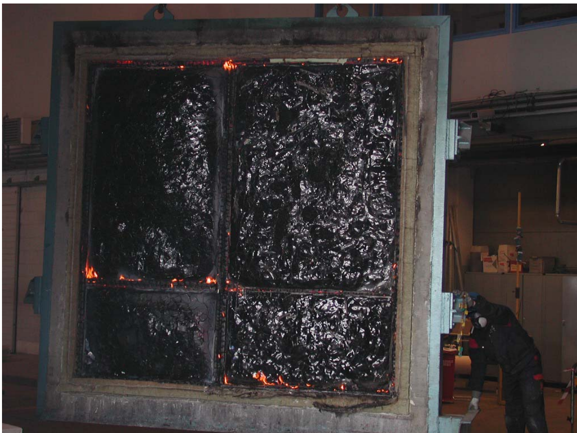
Photo 8: Exposed side of the test specimen after test.
