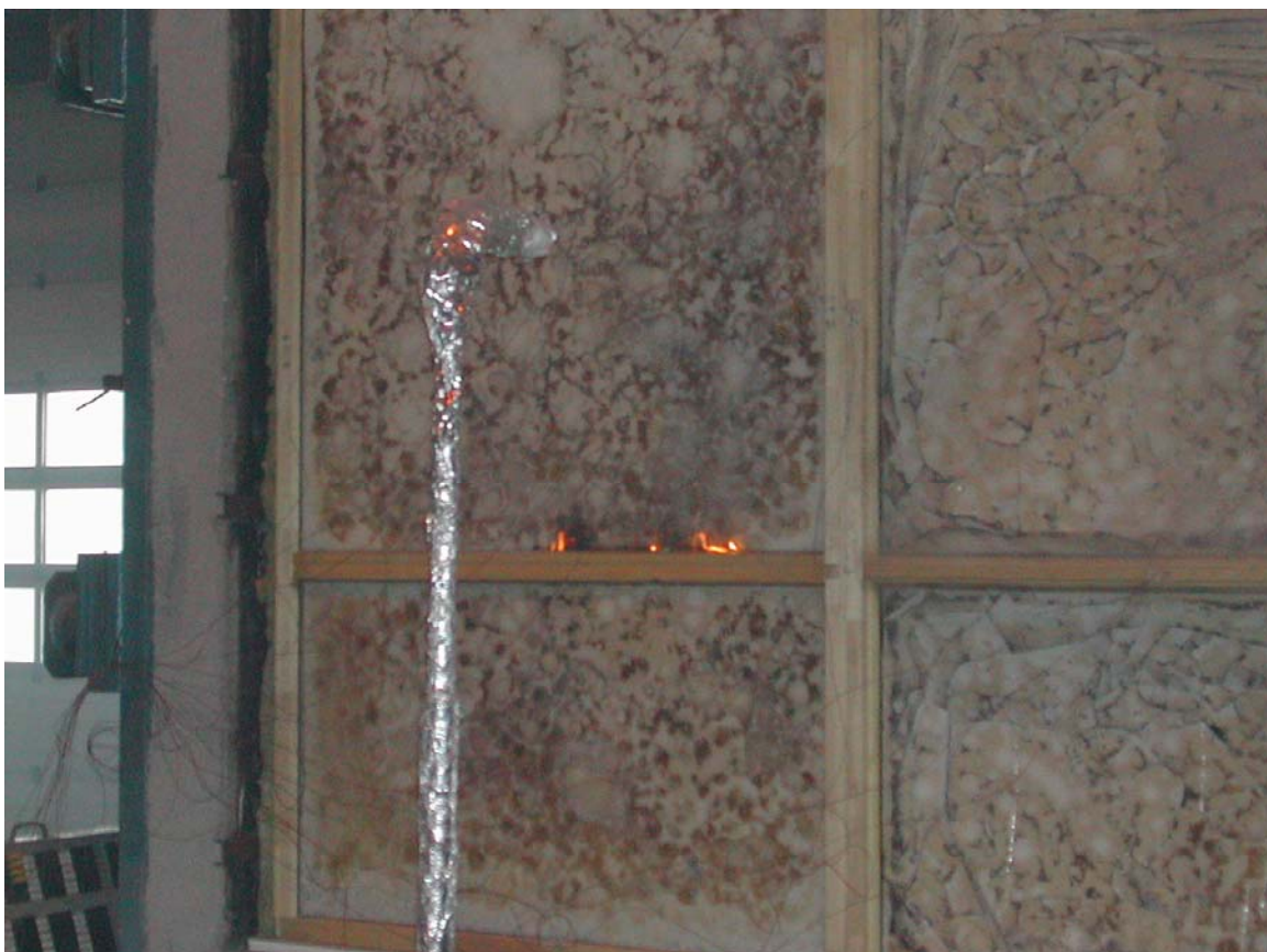
Photo 6: Unexposed side of the test specimen after failure due to sustained flaming.
