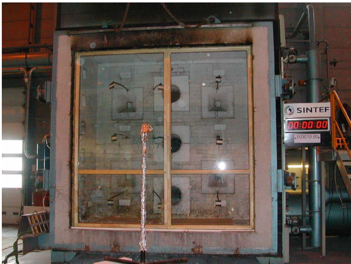
Photo 2: Unexposed side of the test specimen before the fire test.
