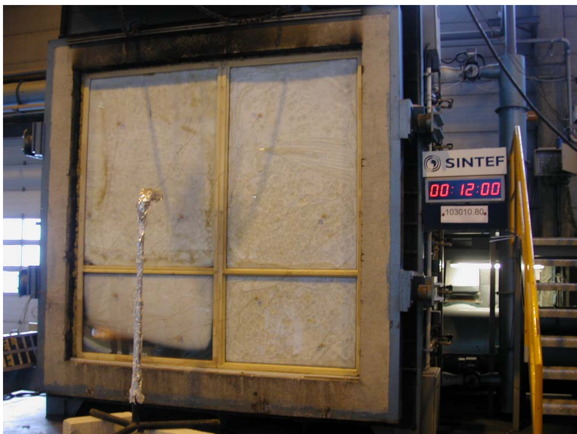
Photo 4: Unexposed side of the test specimen after 12 minutes of fire testing.
